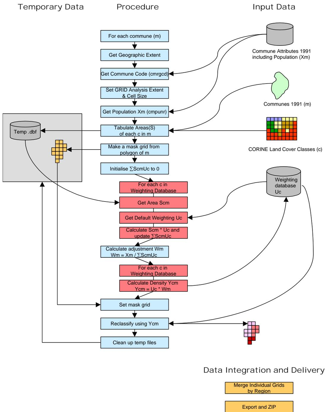
Figure 7 – Algorithm Implementation Workflow
